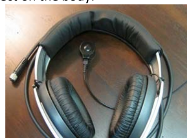
FIGURE 9: BONE CONDUCTOR AND AIR/BONE CONDUCTION HEADPHONES
